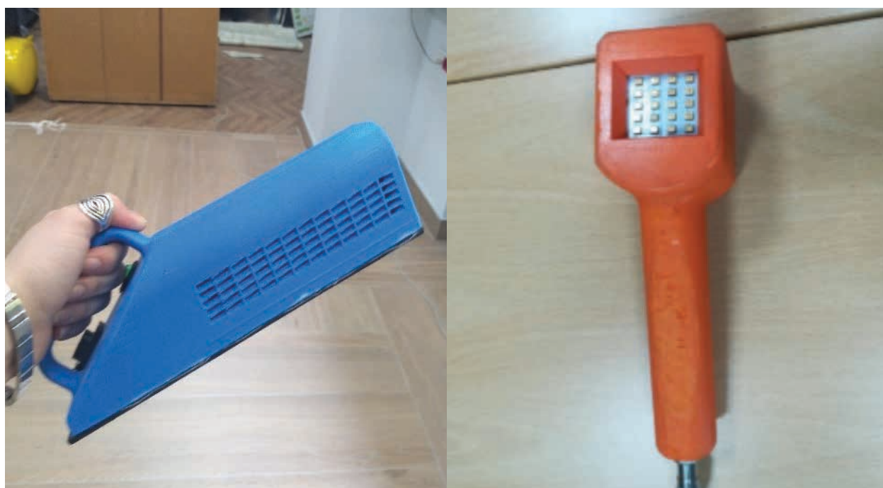
Figure 6 Sterilizer based on the UVC light with a wavelength of 245 nm (left) and Sterilizer based on the UVC light with a wavelength of 275 nm (right) [9]
