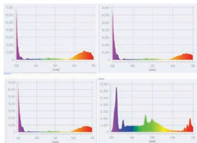
Figure 4: Hyperlight fusion effect: a) spectrum of LED UV radiation ( \lambda=380 nm) with the appearance of the second harmonic in the range of \lambda=680-780 nm. b) The UV radiation spectrum affecting the skin
