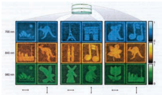
Figure 2.7 The first five-dimensional memory of 1 Tbit/cm 3 , based on the use of three wavelengths and two polarized lights (Zijlstra et al, 2009).
