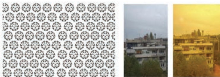
Figure 6.33 Thin film of C_{60} molecules 60 nm – 100 nm thick on a glass scaffold. Distribution of C_{60} molecules in the film. Due to \pi electrons present in each C_{60} molecule, repulsive forces are generated and the molecule rotates freely about 3 \times 10^{10} \text{ s}^{-1} (Koruga, Dj, PCT Patent US2008/0286453 A1, Applicant DVB Global USA).
